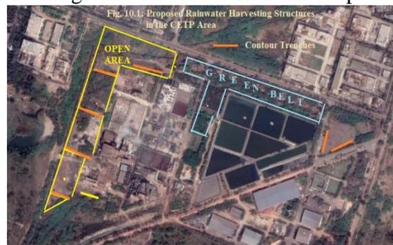
**10.1.1 Trench across slope:** The open area along the west border is about 350m length and 60m width consists of some bushes and plants. The diverted stream on the north border flows along the west border of the site. Five trenches are proposed in the vacant land aligning across the slope. Each trench should be excavated for about 50m to 55m length, 0.5m width and 1.0m depth. Trench should be filled to 3/4th level with permeable material like boulders at bottom,
