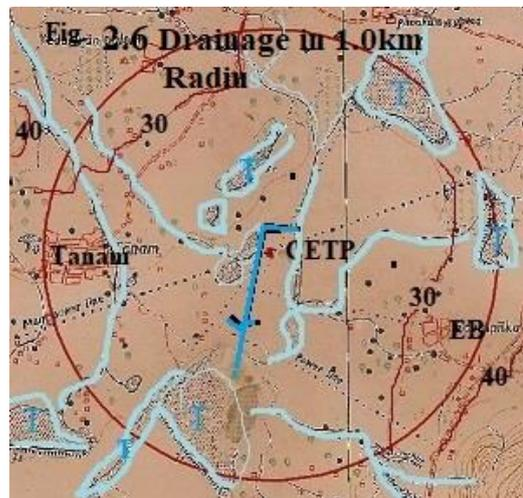
However, a drain is constructed along the north boundary of CETP to divert surface run off from the JNPC main stream catchment as well from the hill slopes of Edullapalli Bonangi from east side. All the runoff/ storm water is diverted through the newly constructed drain towards west direction and at the end point of the CETP site, the drain is along the west boarder of CETP till it reaches a tank which is about 200m distance from southern border as shown in fig.
