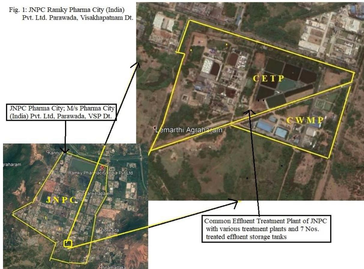
Pharma City (India) Pvt. Ltd. Spread in an area of about 693 Hectares as per the boundary marked in fig. 1.1 Common Effluent Treatment Plant (CETP) is part of JNPC and its area is about 16.6 Hec. as marked above that consists of 9 guard ponds and effluent treatment units.
